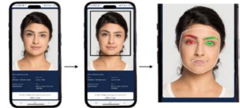
Face detection using Caffe (Deep learning based Face detector)
